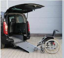
With the unfolded ramp the vehicle can be accessed comfortably with a wheelchair.
